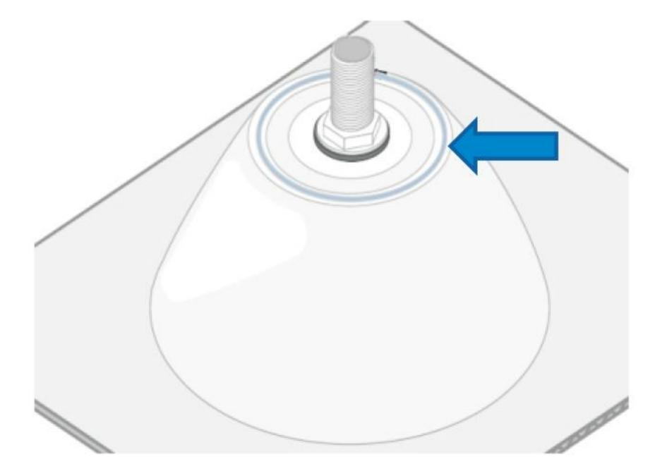
5. Apply the silicone slightly in from the outer edge on the underside of the basin.
